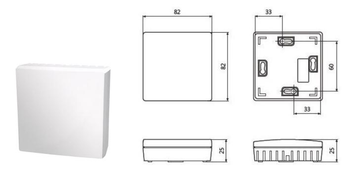
An indoor sensor in modern housing design measures the temperature in the range of -30 up to +60°C in gasiform medium and is with all current sensors available. The temperature probe can be mounted directly on-wall or onto a junction box by 2 fixing screws. The extra wide ventilation slots ensures a good air circulation for a high accuracy of measurement.
